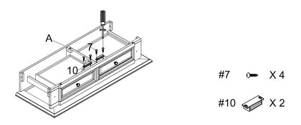
Step 2. Attach door magnets (part #10) to bottom panel (part H) using screws (part #7) and Phillips head screwdriver.
